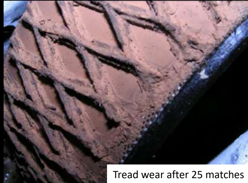
Performance wheel with Roughtop Tread installed.
