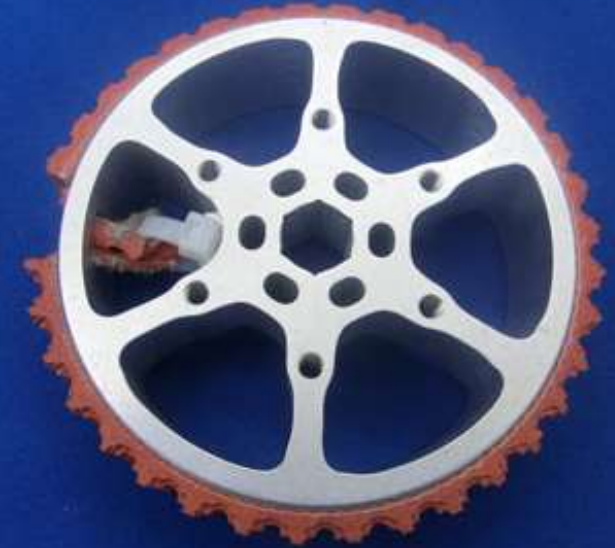
Performance wheel with Roughtop Tread installed.
